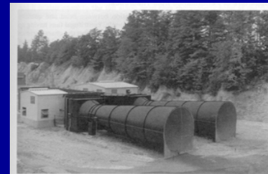
FIGURE 9.4 Axial-flow fans, model 8HU117, dual installation. (By permission from Jeffrey Mining Machinery Division, Dresser Industries, Inc., Columbus, OH).
